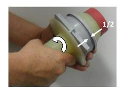
Remove the safety cap from the hole punch. Push the punch firmly into the side of the poly tubing, embedding it up to the half-centimeter gap in the gate valve.
