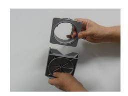
Insert the hole punch into the same side from which the gate was removed, making sure to match up the valve groove with the hole puncher guide groove.
