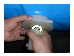
Remove the hole punch and place the gate into the valve again to close.
